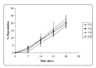
Fig. 4: Degradation studies of the implants F1, F2, F3 and F4, n=3, Data presented as mean±SD
