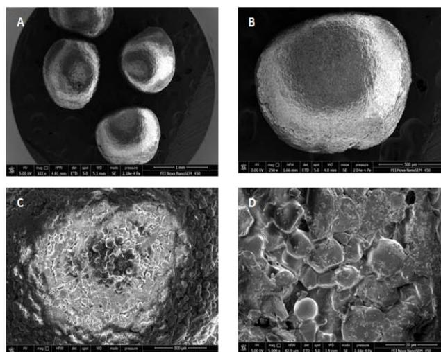
**Fig. 7: SEM images of optimized formulation batch IX; A) at 103X, B) at 250X, C) at 1000X, and D) at 5000 X**
