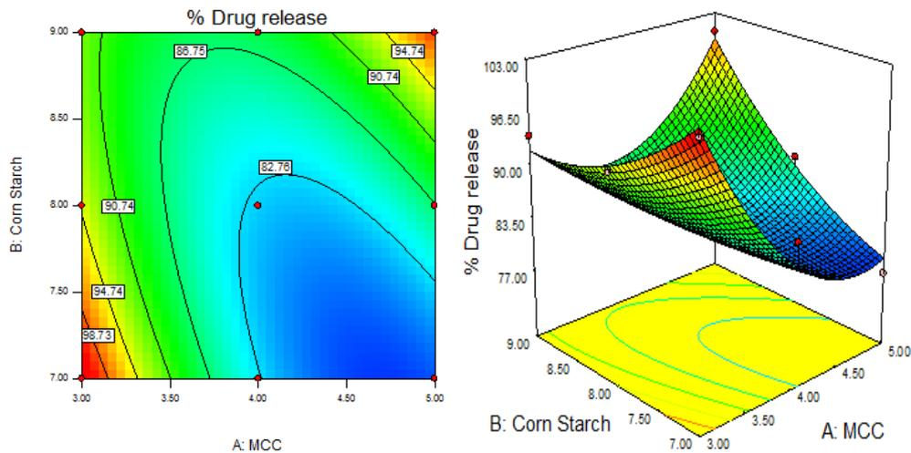
Fig. 4: Different plots showing the effect of independent variables on % drug release of pellets after 10 min, (A) Counterplot showing the relationship between various levels of two independent variables, (B) Response surface plot showing the influence of the concentration of MCC and Corn Starch on the % drug release of pellets after 10 min
