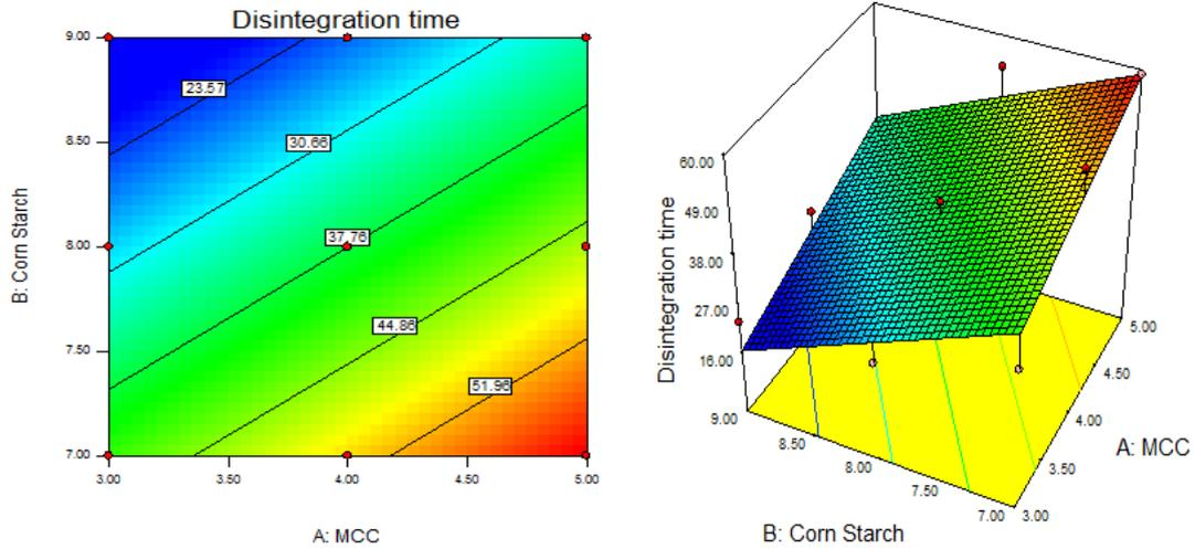
Fig. 3: Different plots showing effect of independent variables on Disintegration time of pellets, (A) Counterplot showing the relationship between various levels of two independent variables, (B) Response surface plot showing the influence of the concentration of MCC and Corn Starch on the Disintegration time
