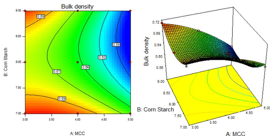
**Fig. 6: Different plots showing the effect of independent variables on the bulk density of pellets, (A) Counterplot showing the relationship between various levels of two independent variables, (B) Response surface plot showing the influence of the concentration of MCC and corn Starch on the bulk density of pellets**
