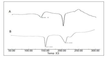
Fig. 1: DSC thermogram of (A) IB and (B) mixture of IB with all excipients
