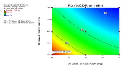
Fig. 4(a): Two-dimensional contour curve of GG ( $X_1$ ) and XG ( $X_2$ ) for %CDR at 18 h ( $Y_2$ )
