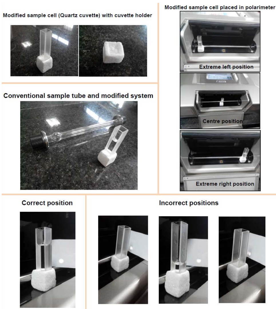
Fig. 1: Photographs of modified instrumentation of polarimetric assay method for small volume samples
