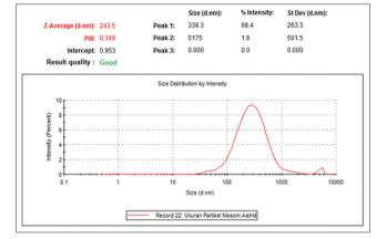
Fig. 4: Size and distribution of niosome particles
