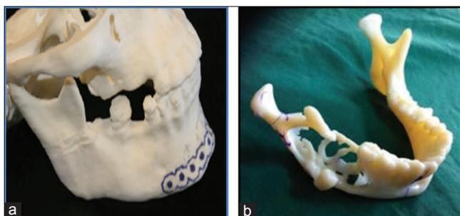
**Fig. 1: (a and b) Example of three-dimensional model made using fused deposition material (FDM) technology with original source data from an multislice computed tomography scan and processed into stereolithography data to be printed using software and produced using an FDM printer [3]**
