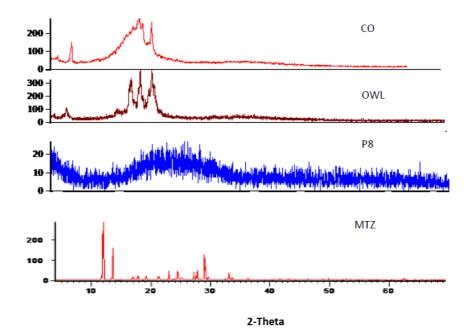
Fig. 2: X-ray patterns of metronidazole (MTZ), coconut oil (CO), ovucire WL (OWL) and the selected pessary (P8)
