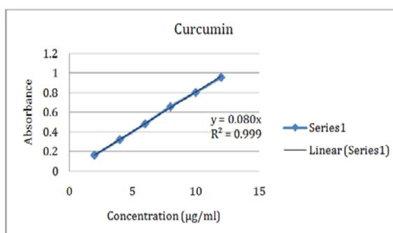
Fig. 7: Calibration curve of curcumin at 425 nm
