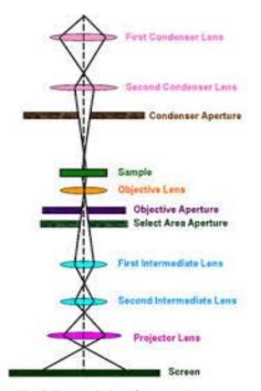
Fig. 5: Transmission electron microscope
