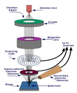
Fig. 4: Scanning electron microscopy
