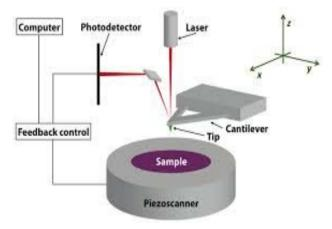
Fig. 6: Atomic force microscopy
