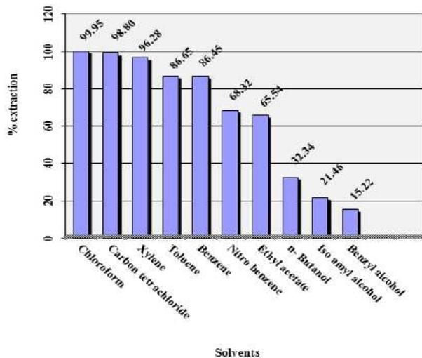
Fig. 2: Effect of solvents on extraction of Fe (III)
