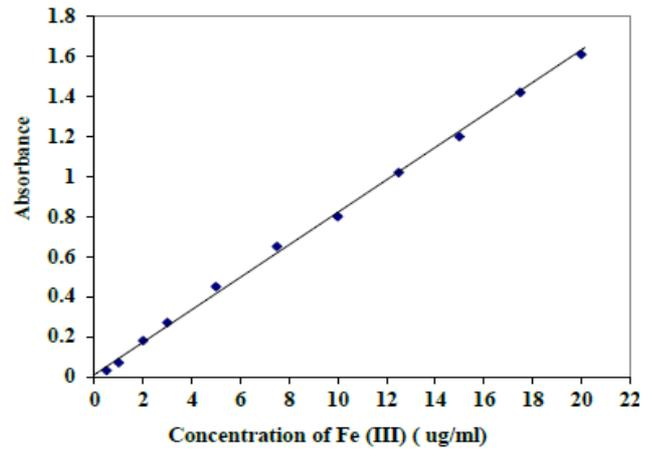
Fig. 4: Calibration curve for iron
