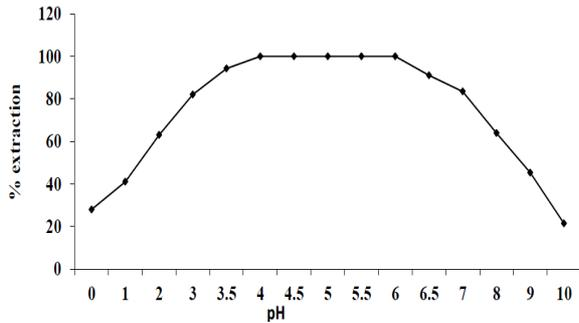
Fig. 1: Effect of pH on the extraction of iron with HOIMNP into Chloroform
