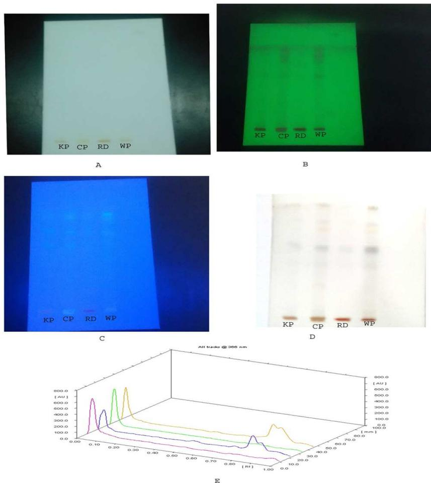
**Fig. 2: Separation of methanol extract on HPTLC Si 60 F<sub>254</sub> with Toluene: Chloroform: Acetone (4:2.5:3.5 V/V), chamber saturation, stained with the vanillin-sulfuric acid reagent. Tracks: 1. KPDR extract, 2. CPDR extract, 3. RD extract, 4. WPDR extract. A-Day light, B-Short UV (254 nm), C-Long UV (366 nm), D-After Visualizing agent. E-3D graph of the respective samples**
