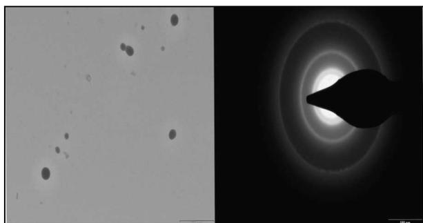
**Fig. 3: TEM analysis of Selenium nanoparticles revealed size of particles 7-48 nm**
