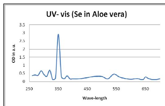
Fig. 2: UV-VIS spectra selenium nanoparticles
