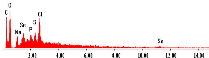
**Fig. 5: EDAX spectrum of selenium nanoparticles**
