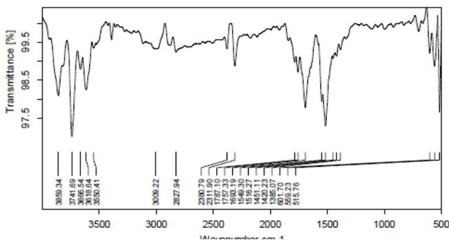
Fig. 3: FT-IR Spectra of MCC
