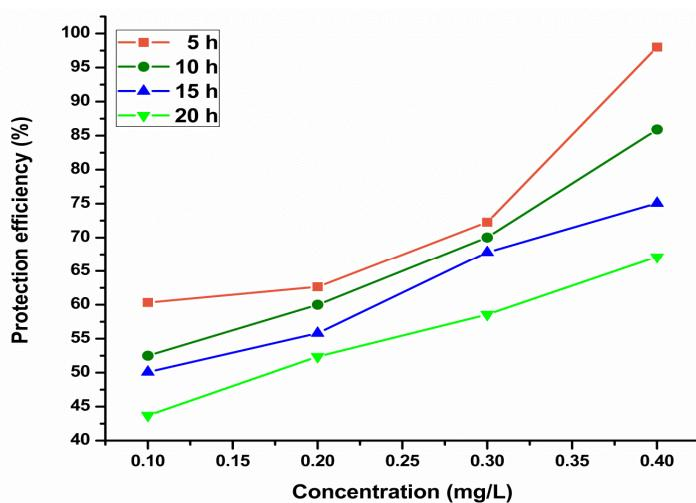
**Fig. 1: Protection efficiency values obtained from weight loss technique**
