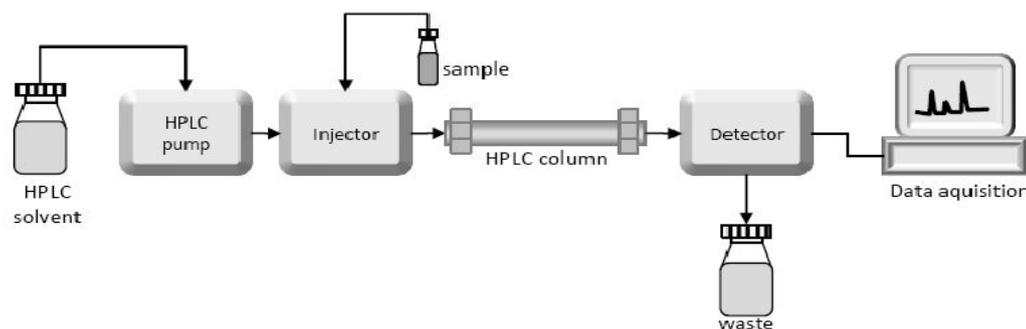
**Fig. 1: Instrumentation of HPLC**
