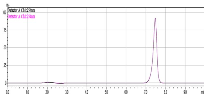
Fig. 20: Chromatogram of salicylic acid (150 ug/ml)
