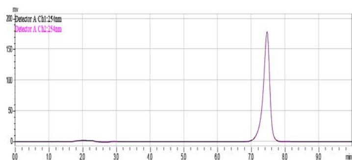
Fig. 21: Chromatogram of salicylic acid (300 ug/ml)
