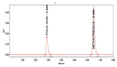
Fig. 19: Typical chromatogram of methotrexate and folic acid
