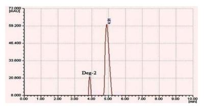
Fig. 29: Chromatogram of phenobarbitone after alkali hydrolysis
