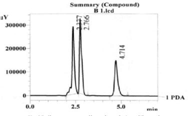
Fig. 25: Chromatogram of base degradation of Ibuprofen
