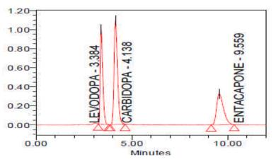
Fig. 10: Standard chromatogram of Levodopa, Carbidopa and Entacapone
