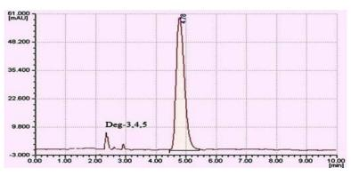
Fig. 30: Chromatogram of phenobarbitone after oxidative hydrolysis
