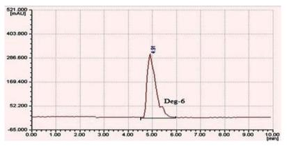
Fig. 31: Chromatogram of phenobarbitone after dry heat degradation
