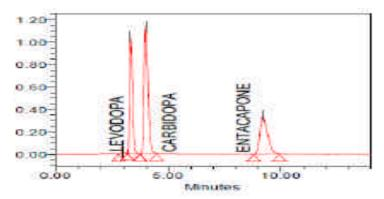
Fig. 12: Chromatogram of acid degradation of levodopa, carbidopa and entacapone
