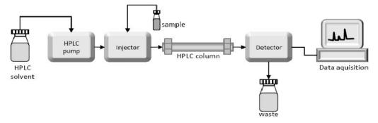
Fig. 1: Instrumentation of HPLC
