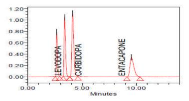
Fig. 14: Chromatogram of alkaline degradation of levodopa, carbidopa, and entacapone
