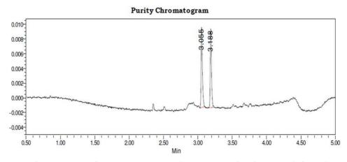
Fig. 7: Typical representative chromatogram of LOD and LOQ of sorafenib and regorafenib drug substances
