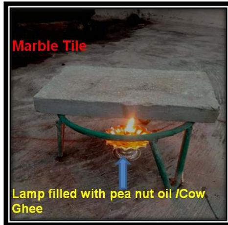
Fig. 2: Preparation of carbon soot by using marble tiles, *Aloe vera* and Ghee/peanut oil
