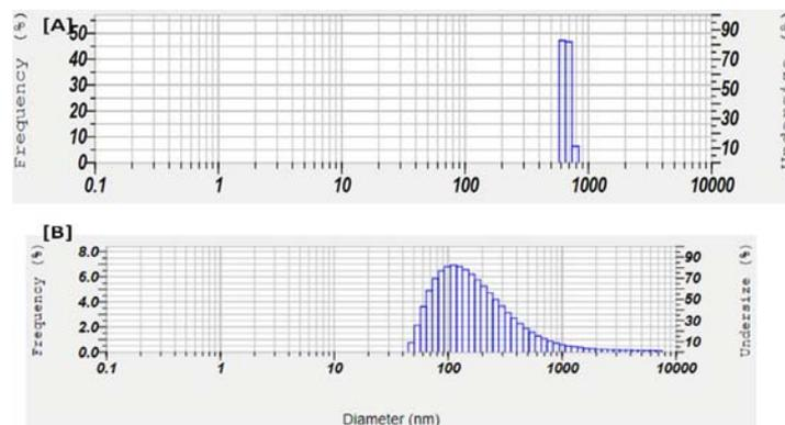
Fig. 2: Zeta-potential and mean particle size graphs of GMS [A] and Beeswax [B] HSLNs
