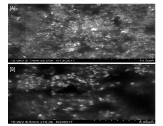
Fig. 1: SEM Images of GMS [A] and Beeswax [B] solid lipid nanoparticles
