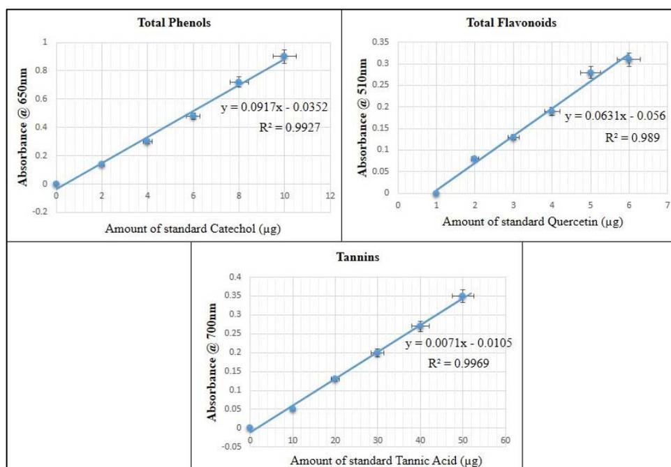
Fig. 2: Standard plots of total phenols, total flavonoids and tannins respectively for the quantification of phytoconstituents
