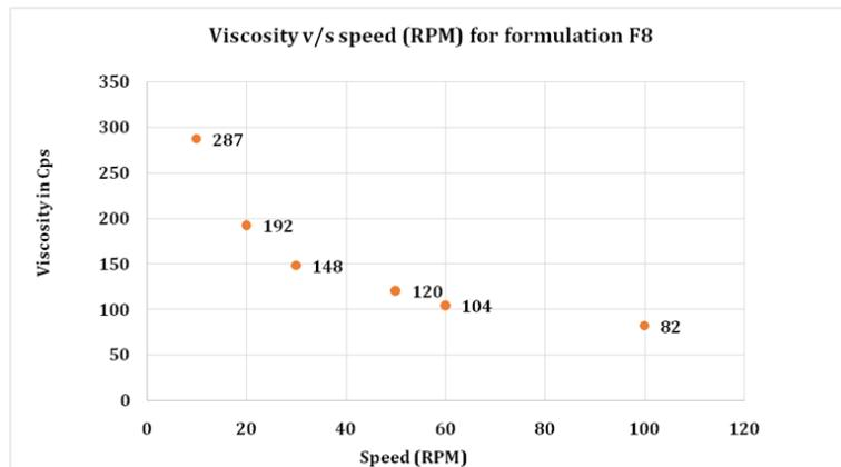
**Fig. 4: Viscosity v/s speed (RPM) for formulation F8**
