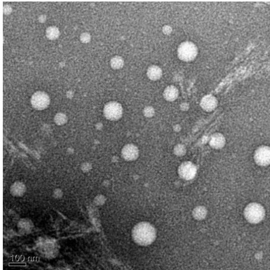
**Fig. 16: Transmission electron microscopy (TEM) Images of optimized SNEDDS**
