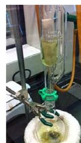
Fig. 1: Soxhlet apparatus
