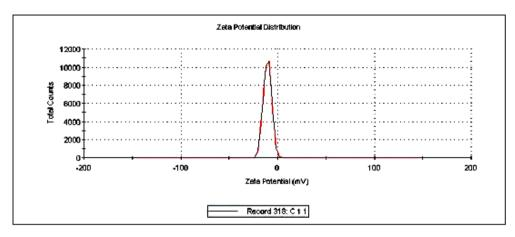
Fig. 7: Zeta potential for optimized batch
