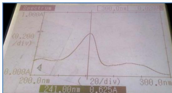
Fig. 2: Zero order derivative of vilazodone HCl
