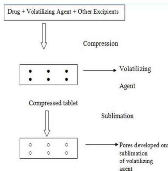
Fig. 3: Schematic diagram of sublimation techniques for preparing fast dissolving tablets [24]
