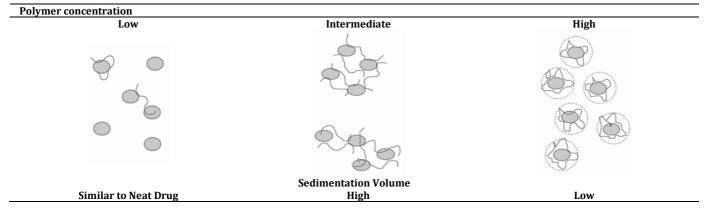
Fig. 5: Flocculation by hydrophilic polymers. The optimal degree of flocculation and sedimentation volume occurs when a large number of interparticle bridges are formed. High concentrations of polymer result in a deflocculated suspension via steric repulsion
