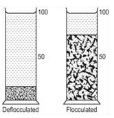
Fig. 1: Schematic representation of deflocculated and flocculated suspension
