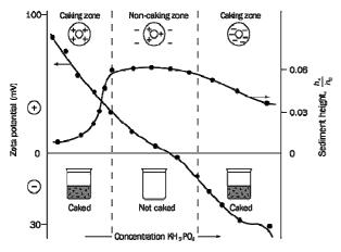
Fig. 4: Typical relationships between caking, zeta potential and sedimentation volume, as a negatively charged flocculating agent is added to a suspension of positively charged particles
