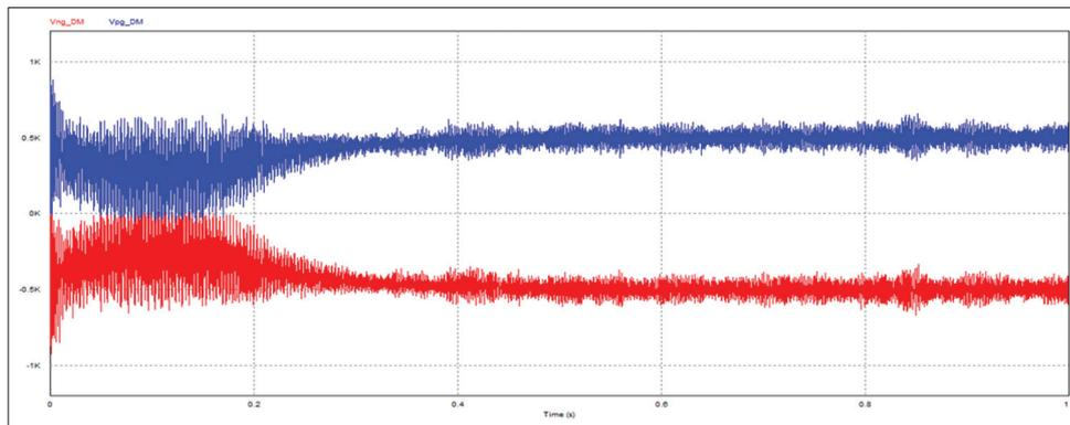
**Fig. 4: DC bus-to-GND voltage in differential mode**
