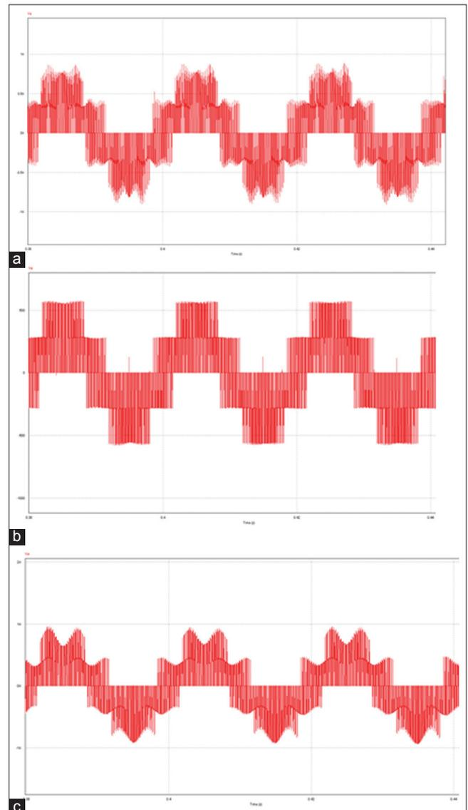
**Fig. 6: AC input-to-GND voltage under different grounding.**
