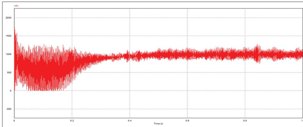
**Fig. 3: DC bus voltage in differential mode**
