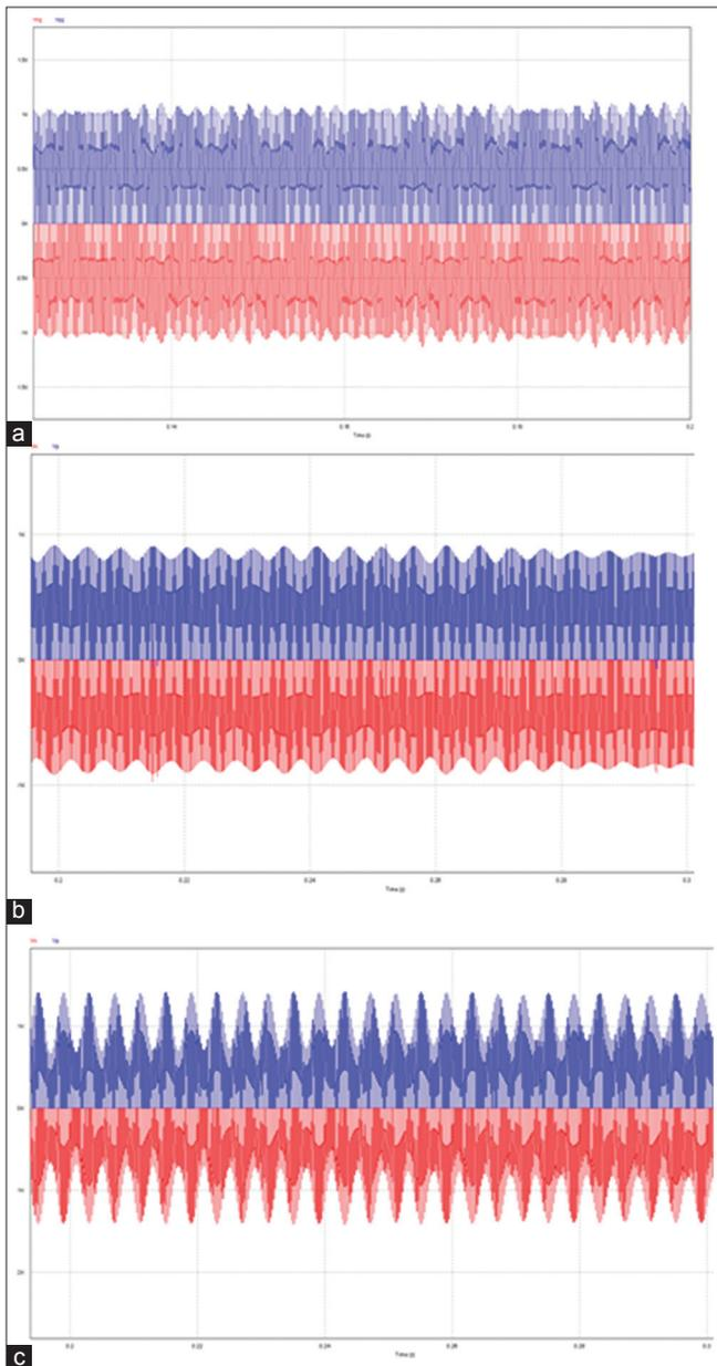
**Fig. 5: DC bus-to-GND voltage stresses under different grounding**
