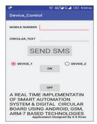
The android application designed, acts as a communication interface between the SIM in GSM module and the user. The interface is quiet user-friendly and easy to access. On opening the application, its homepage provides two functionalities.
