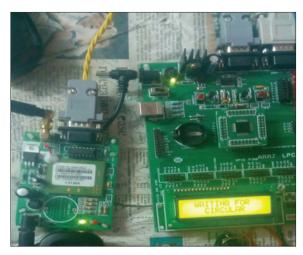
Fig. 3: Interface with global system for mobile module
