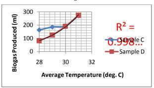
Fig. 3.4: Biogas production variation with temperature.
