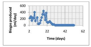
Figure 3.2: Daily Gas Production Rate (ml/day) for sewage concentration of 0.5kg/l using Transparent Plastics as Bioreactors
