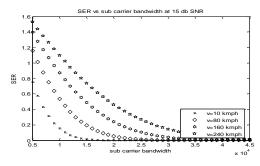
Fig.6: SER vs. Sub Carrier Bandwidth at SNR=15 dB
