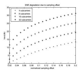
Fig.1: SNR degradation due to sampling offset
