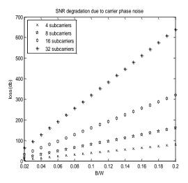
Fig.3: SNR degradation due to carrier phase noise
