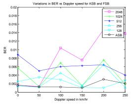
Fig.10: BER comparison of ASB vs. FSB OFDM systems when target BER=0.01.
