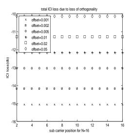
Fig.2: Total ICI loss due to loss of orthogonality
