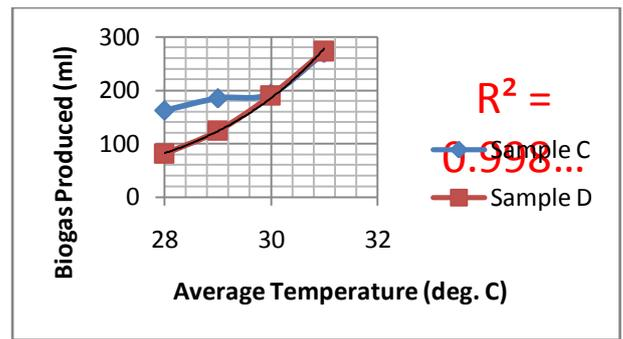
**Fig. 3.4: Biogas production variation with temperature.**
