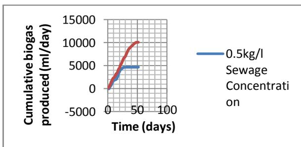
**Fig. 3.3: Cumulative Daily Biogas Production (ml) for Two Different Sewage Concentrations**
