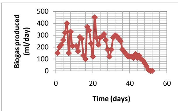
**Figure 3.1: Daily Gas Production Rate (ml/day) for sewage concentration of 0.4kg/l using Transparent Plastics as Bioreactors**
