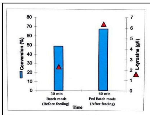
**Fig. 3: Fed batch biosynthesis of L-tyrosine (0.05 M Phenol in batch mode and addition of 0.05 M phenol)**
