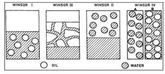
Fig. 1: Phase behavior in accordance with Winsor system
