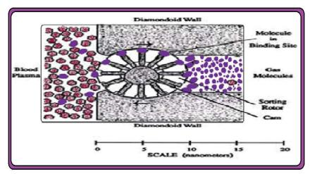
Fig 3: Molecular sorting rotors
