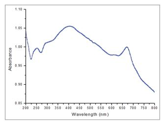
Fig. 3: Ultraviolet-visible spectra of *Solanum villosum* aqueous leaf extract reduction of silver nanoparticles
