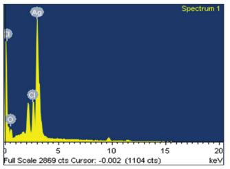
Fig. 5: Energy dispersive X-ray spectrum analysis for biosynthesized silver nanoparticles from aqueous leaf extract of *Solanum villosum*
