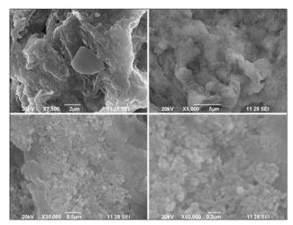
Fig. 4: Scanning electron microscopy micrographs for synthesized silver nanoparticles from aqueous leaf extract of *Solanum villosum*
