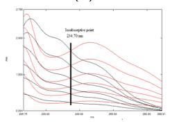
Figure 5: Iso absorptive point at 234.70nm in zero orderspectra (1:1)
