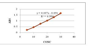
Fig. 8: Calibration graph of Irbesartan at 234.70 nm
