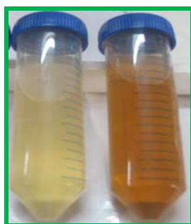
Fig. 1: Light yellow color of the reaction solution containing 2 mM \text{AgNO}_3 and aqueous leaf extract of A. aspera changes to dark brown color after 1 h incubation
