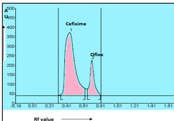
Fig. 6: HPTLC densitogram under optimized conditions showing  $R_f$  value 0.43 for cefixime (40 ng/band) and 0.72 for Ofloxacin (40 ng/band)
