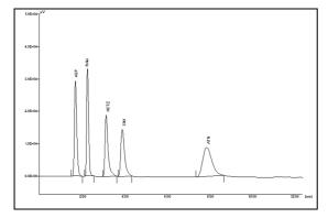
Fig.3: Chromatogram of ASP, RAM, HCTZ, SIM and ATN
