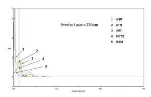
Fig. 2: Overlay Spectrum for ASP, RAM, HCTZ, SIM and ATN (λmax = 230 nm)
