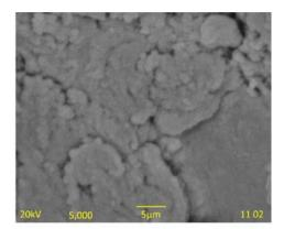
Fig. 3: SEM micrograph of AgNPs synthesized by *T. divaricata* leaf extract.
