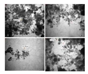
Fig. 4: Transmission electron microscopy images of AgNPs from *T. divaricata* leaf extract with different size distribution.
