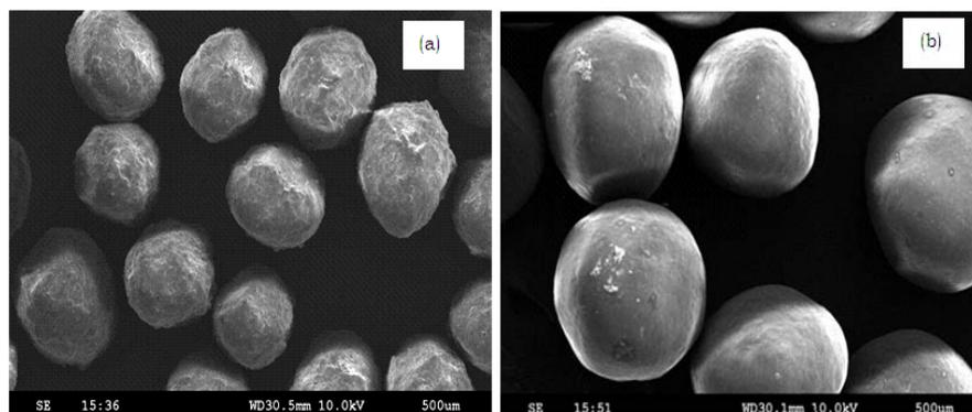
**Fig. 4: SEM pictures of Taste masked pellets with a) 18.75 mg and b) 25 mg Eudragit EPO**
