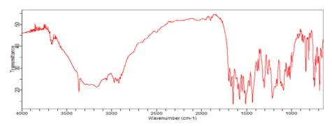
Fig. 4: FTIR spectra of physical mixture of AML and ATR
