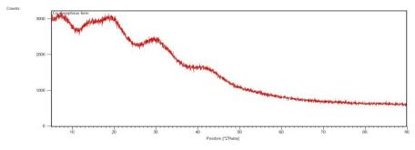
Fig. 10: X-ray powder diffractometer of co-amorphous AML-ATR
