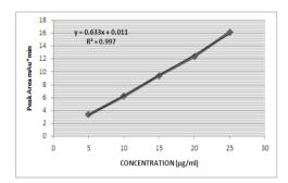
Fig. 2: Calibration Curve of Standard DHA
