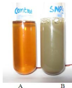
Fig. 1: Synthesis of SNPs: a. Plant extract, b. Plant extract with silver nitrate (SNPs) the color change of leaf extract of Alangium salvifolium
