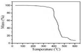
Fig. 2: It shows TGA curve of THQSA resin
