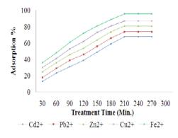
Fig. 3: It shows effect of changing the treatment time on the adsorption % of different metal ions of THQSA resin
