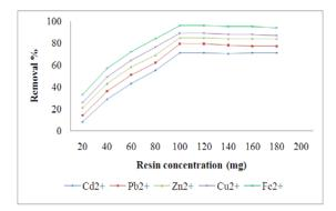
Fig. 5: It shows effect of THQSA resin quantity on removal of metal ions
