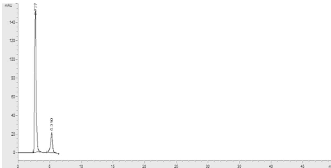
Fig. 4: A typical LC chromatogram of sample solution of prox ( $t_R$  2.73 min) and 8-chlorotheophylline ( $t_R$  5.31 min)
