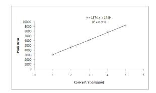
Fig. 5: Calibration curve of Cefoperazone
