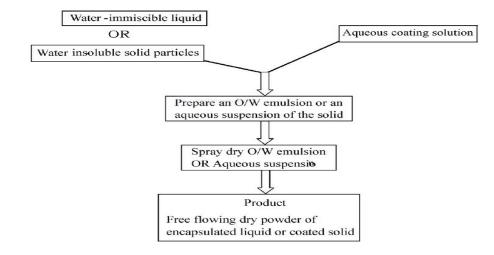
Fig. 1: Flowchart for coating liquid and solid particles using spray-dry process [17]
