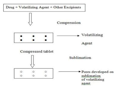
Fig. 2: Schematic Diagram of Sublimation Technique for Preparation of FDT [18]
