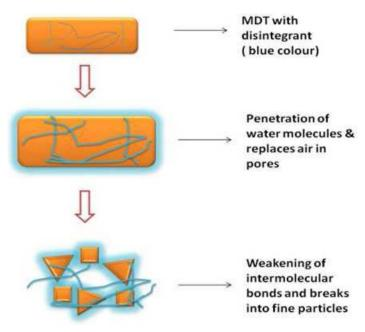
Fig. 1: Wicking mechanism. [26]
